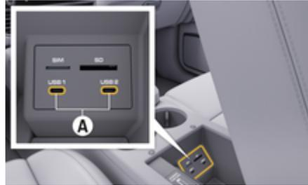
Fig. 2: USB interface (type C) in armrest
