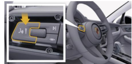
Fig. 4: Voice control button on the control stalk
