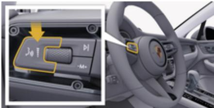
Fig. 13: Voice control button on the control stalk
