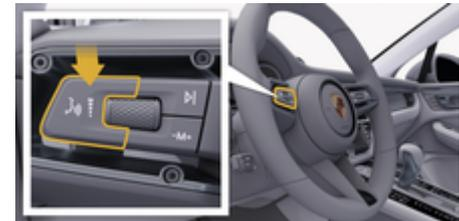
Fig. 3: Voice control button on the control stalk
