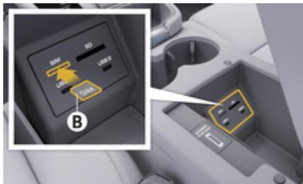
Fig. 1: Insert the external SIM card in the armrest
