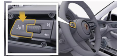
Fig. 10: Voice control button on the control stalk
