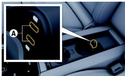
Fig. 3: USB interface (type C) in rear centre armrest
